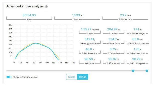
With the Advanced Stroke Analyzer you can view the averages of a segment (part) of the workout and therefore compare them with each other. The R2-Square is the drawn yellow line that could have been the ideal stroke with the values rowed. The blue line is the realized average and you can therefore see the deviation.
